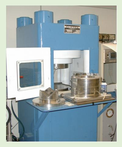
A high pressure/high temperature multianvil press was then used to apply desired conditions to the sample
